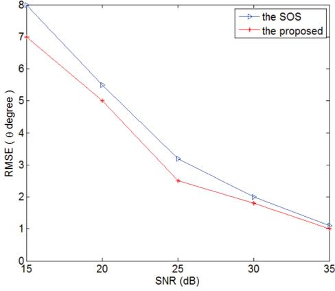
Figure 1: The root mean squared error (RMSE) versus signal-to-noise ratio (SNR)s for the algorithm proposed by Ma *et al.* ( the SOS, as a type of MUSIC ) and the proposed algorithm ( the proposed ) on 100 Monte Carlo trials.
