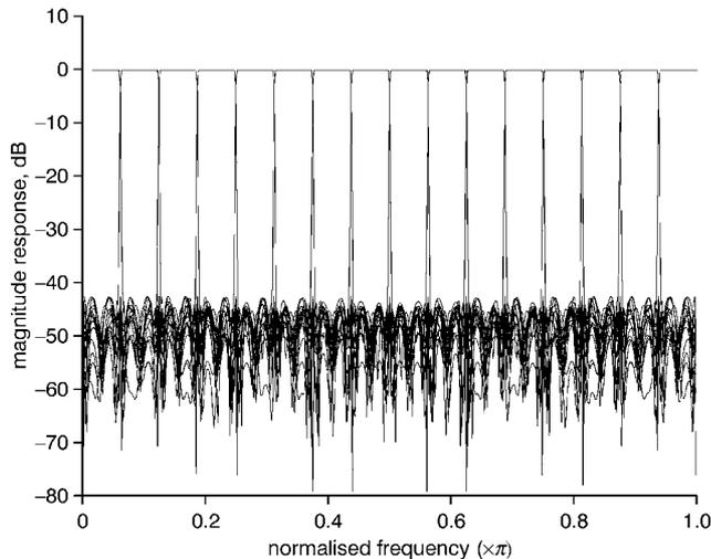
**Fig. 2** Magnitude response of proposed 16-channel IIR CMFB
