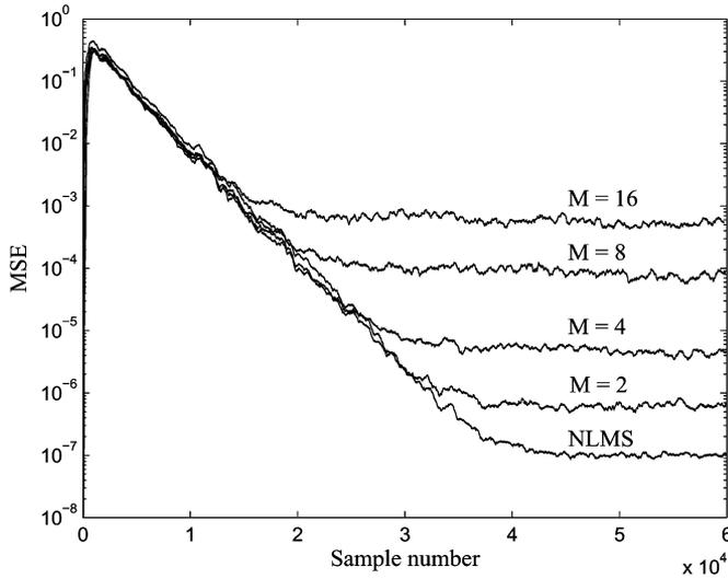
Fig. 8. MSE performance for the proposed SAF algorithm for different values of  $M$  and the fullband NLMS algorithm for a white noise input.
