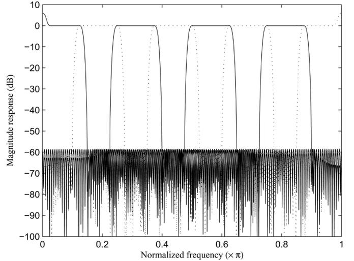
Fig. 7. Magnitude response of the eight-channel bandwidth-increased analysis filters.
