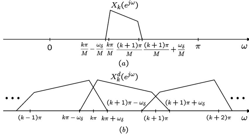
Fig. 3. Magnitude responses of the signals in the  $k$ th subband. (a) Output of the  $k$ th analysis filter. (b) Its downsampled version.
