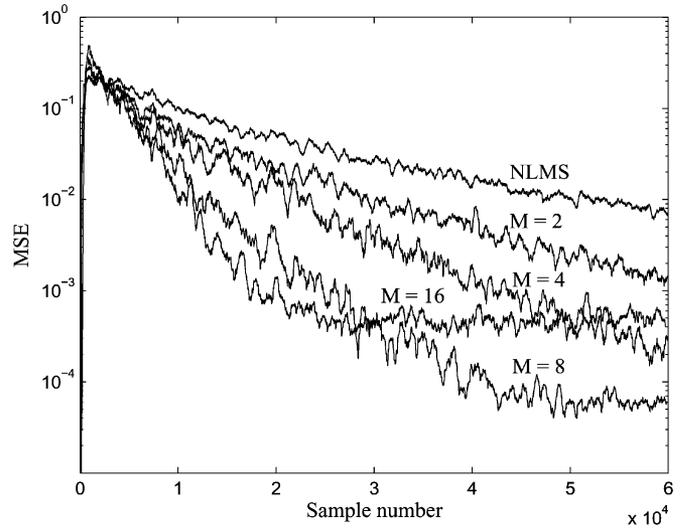
Fig. 9. MSE performance for the proposed SAF algorithm for different values of  $M$  and the fullband NLMS algorithm for a colored input.
