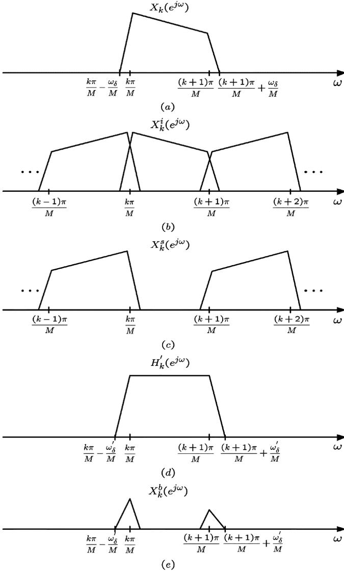
Fig. 5. Magnitude responses of the signals of the proposed SAF structure. (a) Output signal of the  $k$ th analysis filter. (b) Interpolated version of  $X_k^s(e^{j\omega})$ . (c) Resulting signal after subtracting  $X_k(e^{j\omega})$  from  $M \cdot X_k^s(e^{j\omega})$ . (d)  $k$ th bandwidth-increased analysis filter. (e) Extracted interband aliasing component.
