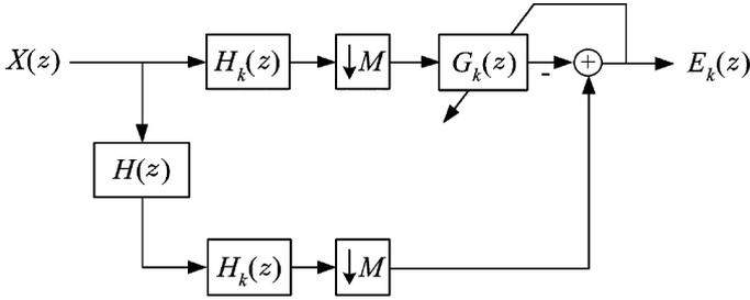
Fig. 1. Block diagram of the adaptive filtering in the  $k$ th subband.  $X(z)$ ,  $H(z)$ ,  $H_k(z)$ ,  $G_k(z)$ , and  $E_k(z)$  represent the  $z$ -transforms of input, unknown system, the  $k$ th analysis filter, the  $k$ th adaptive filter, and the  $k$ th error signal for  $k = 0, 1, \dots, M-1$ , respectively.
