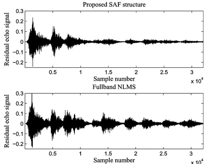
Fig. 10. Residual echo signals using the proposed eight-channel alias-free SAF algorithm and the fullband NLMS algorithm for speech input.
