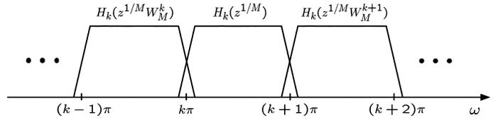
Fig. 2. Magnitude responses of  $H_k(z^{1/M})$  and its adjacent terms  $H_k(z^{1/M} W_M^k)$  and  $H_k(z^{1/M} W_M^{k+1})$ .
