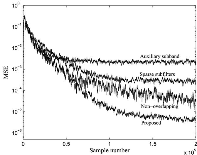
Fig. 11. Comparison of the performances of the proposed alias-free SAF algorithm and the conventional SAF algorithms for a colored input when  $M = 4$ .
