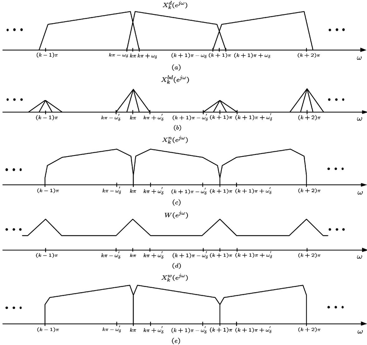
Fig. 6. Magnitude responses of the signals of the proposed SAF structure. (a) Subband input with interband aliasing. (b) Downsampled version of the extracted interband aliasing component. (c) Almost alias-free subband input. (d) Filter for the spectral flatness of the almost alias-free subband signal. (e) Almost alias-free subband input with the flat spectrum.
